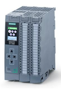
SIMATIC S7-1500 compact CPU CPU 1511C-1 PN, Central processing unit with work memory 175 KB for program and 1 MB for data, 16 digital inputs, 16 digital outputs, 5 analog inputs, 2 analog outputs, 6 high-speed counters, 4 high-speed counters for PTO/PWM/frequency output 1st interface: PROFINET IRT with 2-port switch, 60 ns bit performance, incl. push-in front connector, SIMATIC Memory Card required
