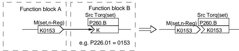
Fig. 3-9 Connecting two function blocks
