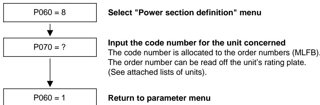
*Fig. 4-2 Sequence for performing the power section definition*
