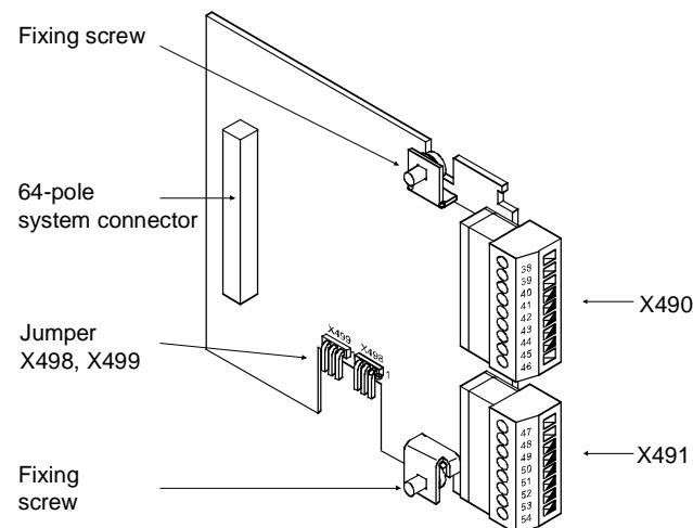
Fig. 2-2 View of the EB2 optional board
