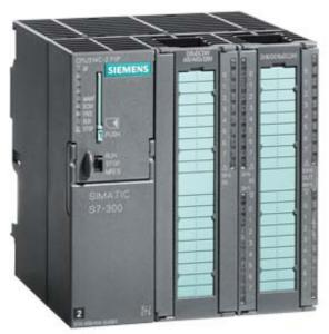
SIMATIC S7-300, CPU 314C-2 PTP COMPACT CPU WITH MPI, 24 DI/16 DO, 4AI, 2AO, 1 PT100, 4 FAST COUNTERS (60 KHZ), INTEGRATED INTERFACE RS485, INTEGRATED 24V DC POWER SUPPLY, 192 KBYTE WORKING MEMORY, FRONT CONNECTOR (2 X 40PIN) AND MICRO MEMORY CARD REQUIRED
